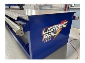
Automated Layout Technology is a pioneer in the automated marking machine arena. ALT designed and developed the Lightning Rail\*, which is the first automated marking machine created specifically for the layout of commercial handrails.
